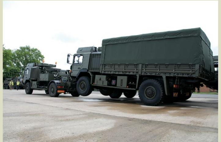
As theatres of operation continue to evolve, EKA Limited foresee a lightweight, highly mobile, towing and intimate recovery requirement for small and medium vehicles. The EKA Lightweight has been developed to address future requirements, where high mobility and manoeuvrability are required, in conjunction with the proven capability of a suspend tow recovery system.
